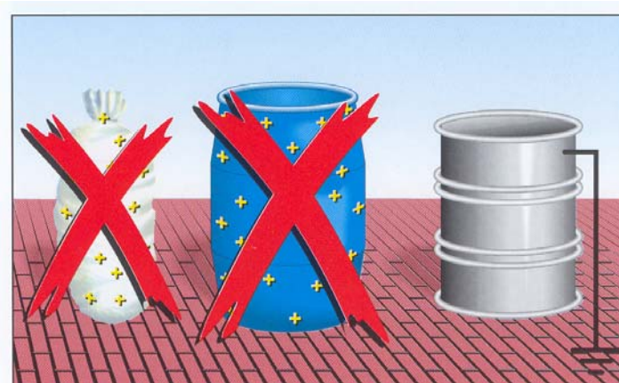
Fig. 2 Avoid electrostatic charges: use conductive, earthed packaging materials (do not use plastic sacks or plastic containers) [1]
